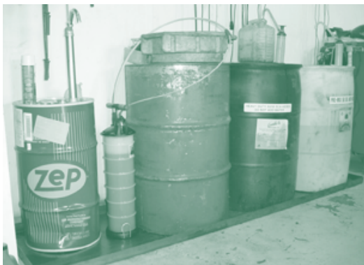
Madrona Autoworks designed and fabricated this spill pan to contain minor spills or leaks of oils, coolant and solvents stored inside their automotive repair business.
