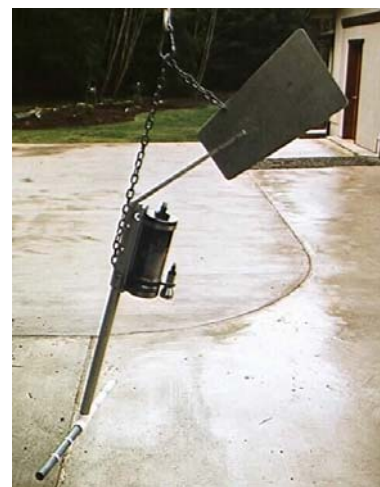
Figure 2. Camera fixture used to video benthic conditions in Totten Inlet.
