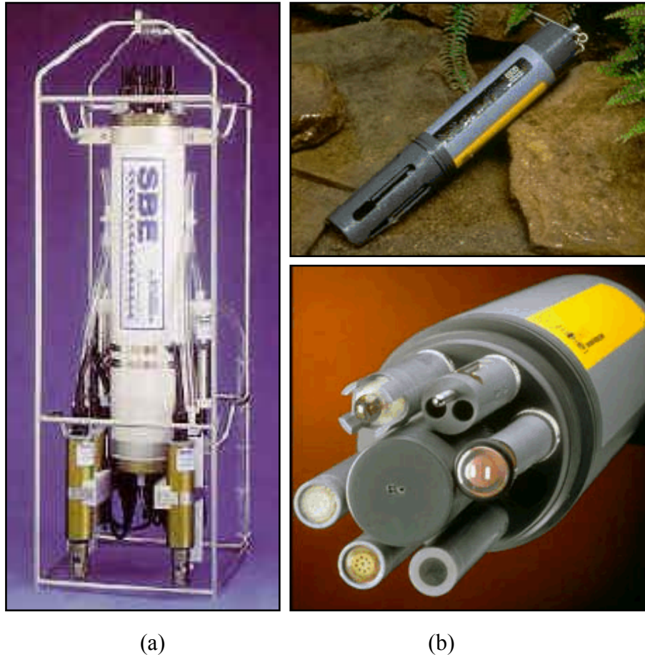
Figure 8: (a) Profiling CTD, (b) Multi-Parameter Sonde (courtesy of Seabird Electronics, Inc. and SonTek/YSI, Inc.)
