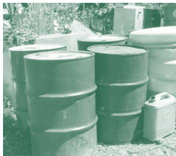
Containers of hazardous materials pose a risk to water resources and public health when stored outside with no secondary containment. Spills or leaks can flow directly into the soil or local water bodies.
