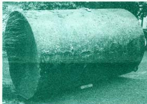
A leaking diesel underground storage tank removed from a local business site.
