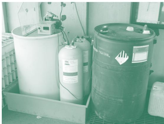
Silver recovery units, like this one at HazoHouse, remove silver from waste fixer before the treated waste can be disposed.
